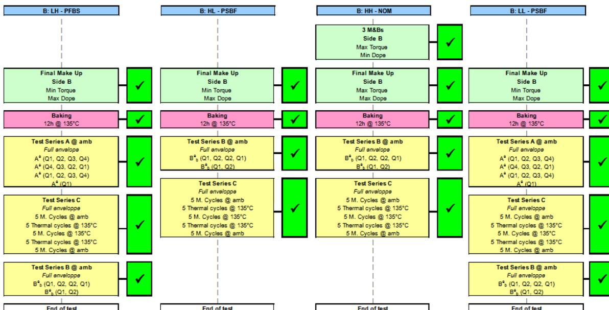
Figure 9. Validated testing protocol according to ISO13679:2002 – CAL III (including customer requirements).
