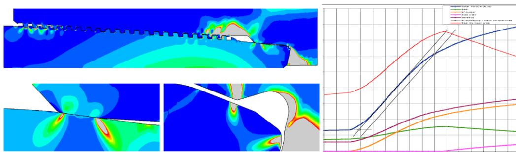
Figure 3. Connection behaviour analysis using FEA for the 10 3/4" 85.3# HW-NA
