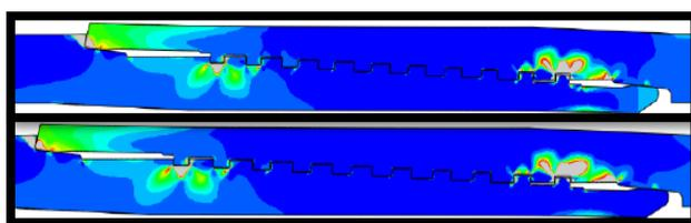
Figure 7. ISOCOLOR representation of one flush connection design – 80ksi (up picture above) & 125 ksi (down picture above).
