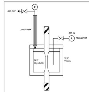
*Figure 2: Test Equipment for Method A—NACE Standard Tensile Test*
