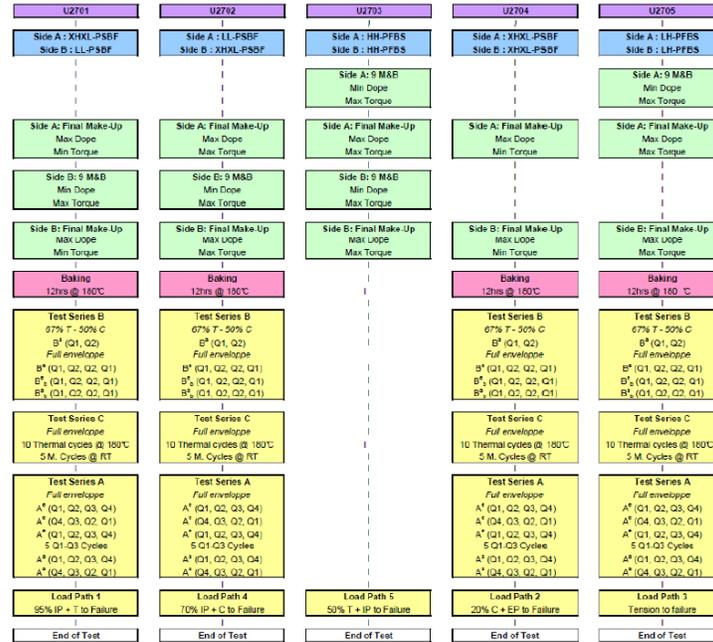
Figure 10: ISO13679:2011FDIS CAL IV testing sequence
